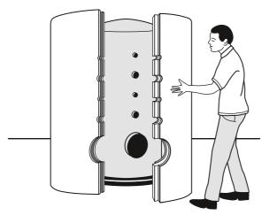
3 Fasten main connection of the insulation
