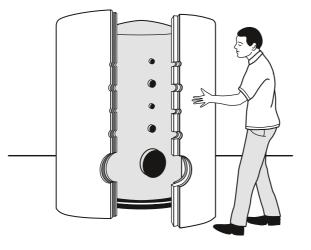
3 Fasten main connection of the insulation
