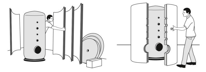
3 Fasten main connection of the insulation
